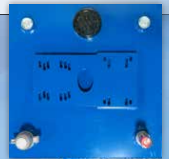
SSW200A Tank Plus Package Shows Top of Tank with Built-In Reel Bracket, (1) 4" NPT Opening, (4) 2" NPT Openings with Lockable Fill Cap with Vent & Fluid Level Gauge.
